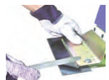
Sharpening with a fine-toothed file
