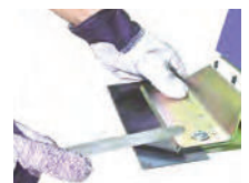
Sharpening with a fine-toothed file
