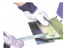
Sharpening with a fine-toothed file
